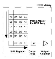
Figure 11. Array Terms for a CCD with a Single Output Amplifier
